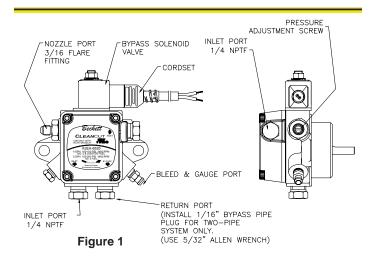
MOUNTING POSITION Beckett CleanCut fuel unit may be mounted in any position (except upside-down during single pipe installation).
