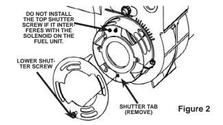
Remove the shutter tab by using a pair of side cutter pliers and file sharp edges flush with burner surface. This will permit the shutter to be locked securely.
